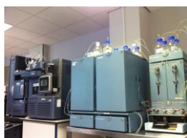
Figure 2: Preclinical method set up Waters Xevo TQ-S interfaced with Spark Holland Symbiosis
