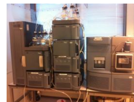
Figure 4: Clinical method set up Waters Xevo TQ-S interfaced with Waters 2D-UPLC.
